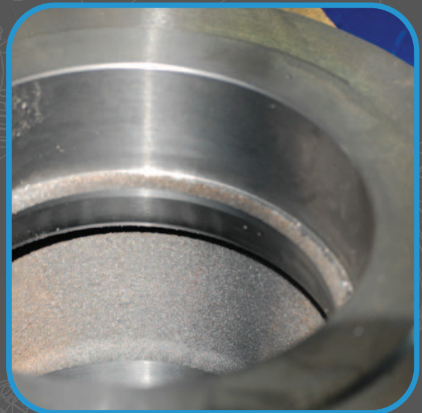
A 316L stainless steel machine welded seat ensures no leak through under the seat as you will often see when the seat is pressed in.
