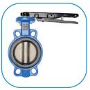
Lug / Wafer PTFE Seated Butterfly Valves Our Av-Tek® lug / wafer PTFE seated butterfly valves come standard with a ductile iron body, 316 SST disc, 420 SST shaft, field replaceable seat, and two piece body for accessibility. Our current offerings are available in sizes 2" -12" and up to 150 psi
