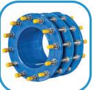
Av-Tek® offers a dismantling joint in a ductile iron body with blue fusion bonded epoxy coating or stainless steelbody. Tie-bars are offered in galvanized or stainless steel.6" -108" sizes available.
